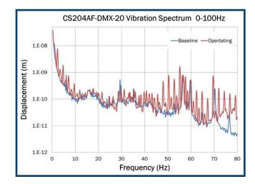
The cryocooler is mounted on an independent structure, dissipating its vibrations to the floor instead of the optical table.
